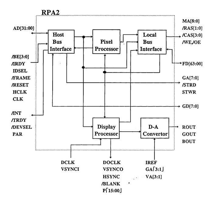
◆ Host Bus Interface = PCI, VL bus compatible interface
