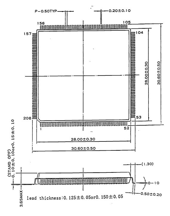
The dimension in parentheses is for reference only. The mold external dimensions do not include flash. UNIT: mm
