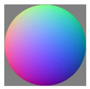
This particular map represents a hemisphere. Each texel on the map is an RGB-encoded vector that corresponds to a unit vector from the origin. Note the corners of the square are grey (0x00808080) which is the RGBA encoded version of the zero vector < 0,0,0 >. There is a small amount of noise generated for visual interest.
